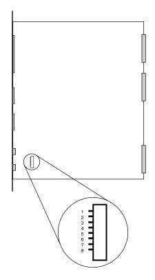
Figure 2-3. Location of Module DIP Switch
